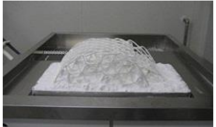
Figure 17 / SLS 3D Printing; laser is used to solidify and bond grains of plastic, ceramic, glass, metal or other materials into layers to produce a 3D object.
