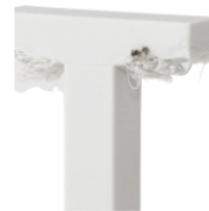
Without support, FDM deposits material in the air and fails to print the letter T
