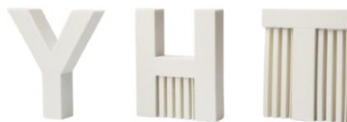
Models of Y, H and T printed with supports by an FDM printer
