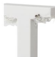
Without support, FDM deposits material in the air and fails to print the letter T
